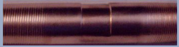
Wear at Support
